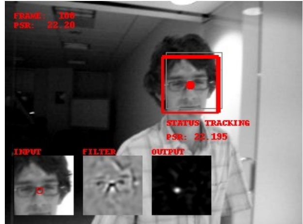
Figure 8: This shows a sample from the dauidin300 sequence for the MOSSE filter. The frame number and PSR are shown in the upper left hand corner. Thin gray box around the face shows starting location of the tracking window for each frame. The thick red box shows the updated location of the track window. The red dot shows the center point of the tracking window and helps to determine if the windows has drifted off the original location. In the Taz video, failure detection is enabled and a red X is drawn in the window to indicate that a failure or occlusion has been detected. Across the bottom of the video are images are the input (cropped from the grey rectangle), the updated filter from this frame, and the correlation output.
