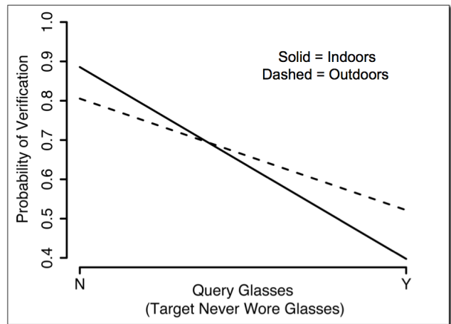
Figure 7. Estimated probability of successful verification for indoor and outdoor query images for cases when the subject did or did not wear glasses in the query image. Note subjects never wore glasses in the target images.
