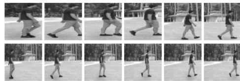
Figure 2. Example tracklet created without (top) and with (bottom) stabilization strategy. Top tracklet uses the bounding rectangles from the track to clip tiles from the source. Bottom uses the full spatial extent of the track within the temporal window to define a single clipping region, and thus stabilizes the images and corrects for minor track drift. In both cases, the clipped tiles are rescaled to fit the fixed tracklet dimensions.
