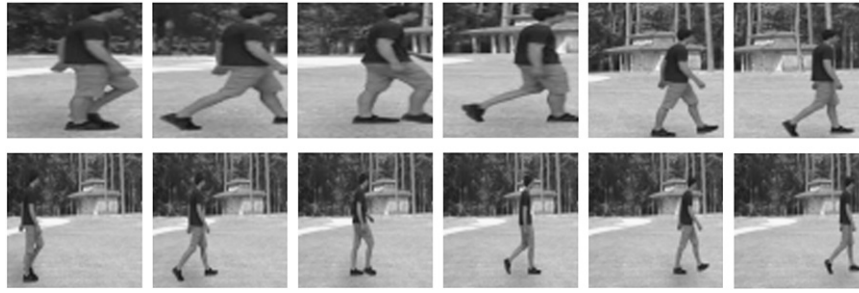
Fig. 10. Example tracklet created without (top) and with (bottom) stabilization strategy. Top tracklet uses the bounding rectangles from the track to clip tiles from the source. Bottom uses the full spatial extent of the track within the temporal window to define a single clipping region, and thus stabilizes the images and corrects for minor track drift. In both cases, the clipped tiles are rescaled to fit the fixed tracklet dimensions.
