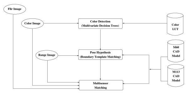
Figure 4: Overview of the ATR Algorithm
