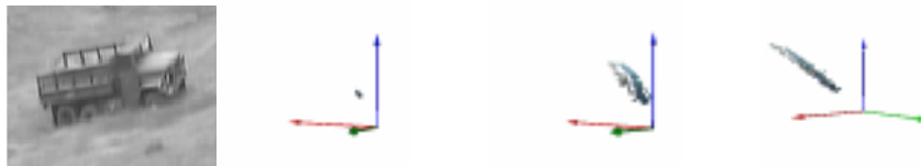
Figure 2: (From left) Sample target; Target color ( RGB ) in a single outdoor image (sample extracted from vehicle hood); Variation of apparent color over several hundred images in a single day; Variation distribution rotated.
