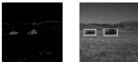
Figure 4: Post-classification binary image (left), with target boundaries extracted (right).
