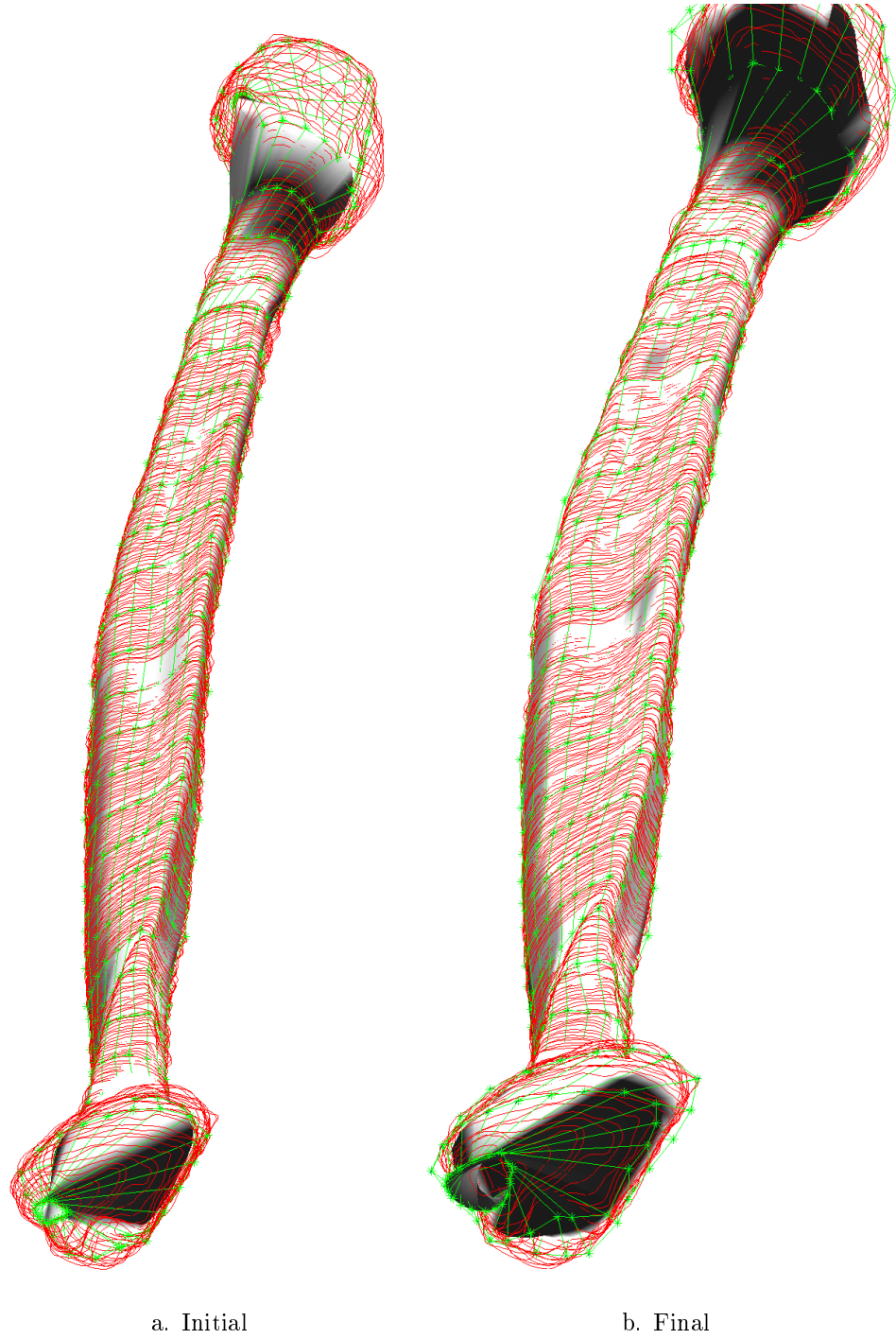
Figure 3: a) Initial NURBS surface (gray) approximating contour data (red) with initial grid of control points (green). b) NURBS surface (gray) after 20 iterations of gradient-descent optimization. The initial control points (red) have been moved to their final positions (green).
