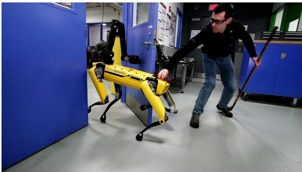
Figure 1: Opening a door by the Boston Dynamics robot. Notice multiple closed chains formed by the legs, arm, and the door.
