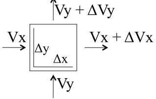
In X direction: cell receives heat VxΔy, loses heat (Vx+ΔVx) Δy, hence ΔVx Δy heat removed
