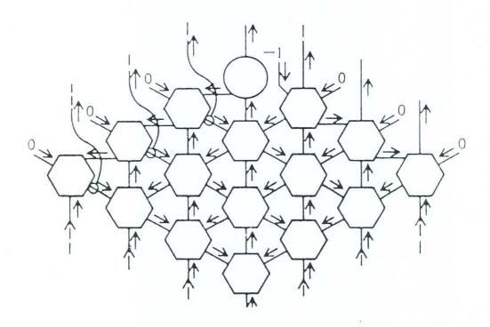
Figure 7-3: Derived Architecture for LU Decomposition
