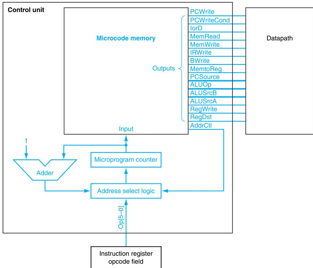
**FIGURE D.4.6 The control unit as a microcode.** The use of the word “micro” serves to distinguish between the program counter in the datapath and the microprogram counter, and between the microcode memory and the instruction memory.
