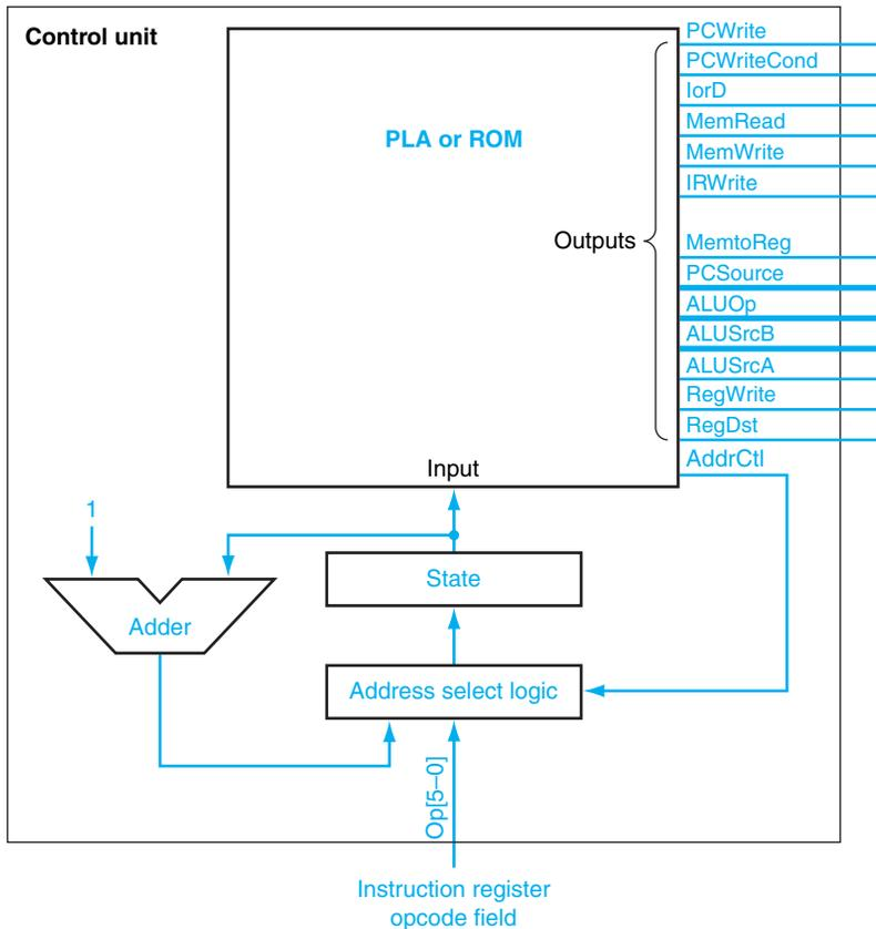
**FIGURE D.4.1 The control unit using an explicit counter to compute the next state.** In this control unit, the next state is computed using a counter (at least in some states). By comparison, Figure D.3.2 encodes the next state in the control logic for every state. In this control unit, the signals labeled *AddrCtl* control how the next state is determined.
