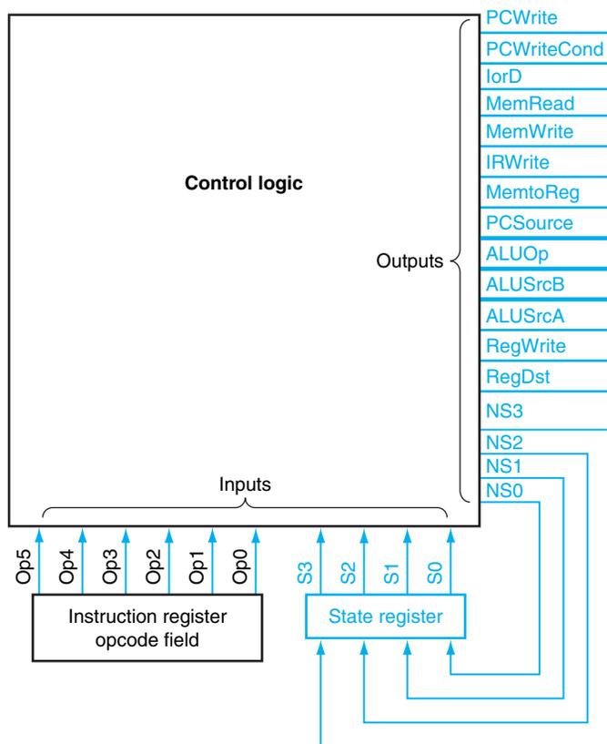
**FIGURE D.3.2** The control unit for MIPS will consist of some control logic and a register to hold the state. The state register is written at the active clock edge and is stable during the clock cycle.
