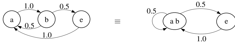
Figure 1.2: Overview model of a system with two useful states and an error state
