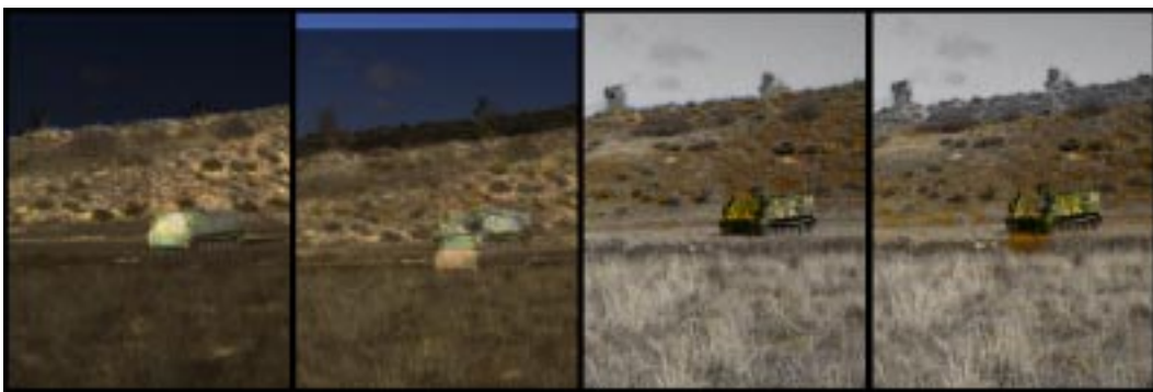
Figure 6: Color To FLIR Relationship. The left-most image shows the FLIR mapped to the intensity component of the color image for the correct transformation. Next, the same mapping is used, but the transformation is incorrect. The final two images show the FLIR mapped to the color saturation component for both the correct and incorrect transformations.
