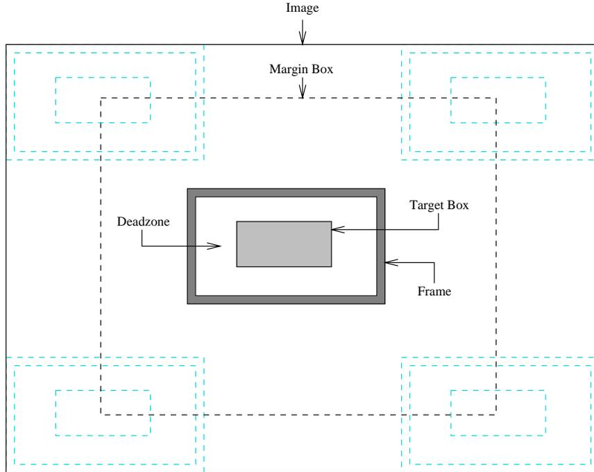
Figure 1: Layout of the components of the sliding detection box.
