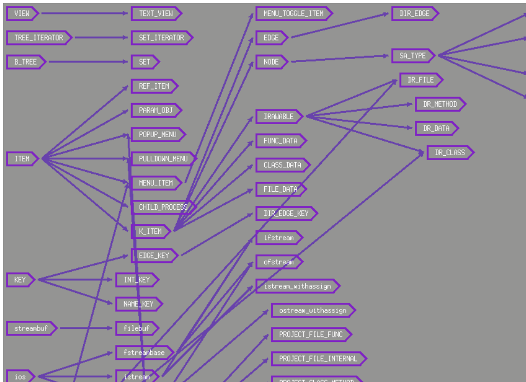
Figure 24: Part of the class-graph produced by SoftBench for CIV.
