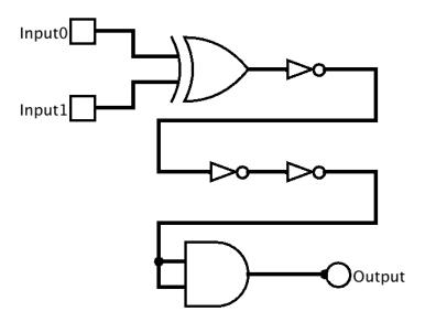
2) Which output signal is asserted for all possible values for Input1 (most significant) and Input0 (least significant) in binary order 00, 01, 10, 11?
