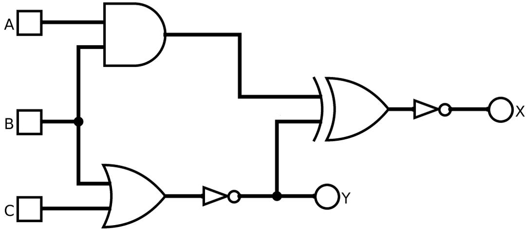
2) Find truth table values by manually toggling the input values and examining the output values. This is done in Logisim by selecting the hand icon and then clicking on each input. Fill in the rest of the truth table for the circuit manually:
