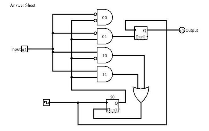
Note that an optimized circuit could do without three of the AND gates pictured above!
