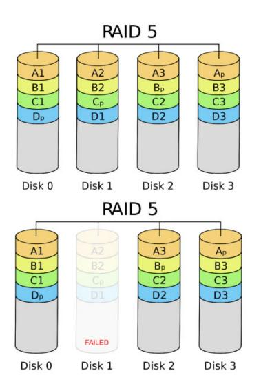
Time to rebuild depends on disk capacity and data transfer rate
