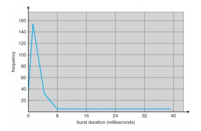
Typical distribution of CPU bursts. Most CPU bursts are just a few ms.
