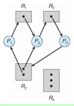
At this point, two minimal cycles exist in the system:  $P1 \rightarrow R1 \rightarrow P2 \rightarrow R3 \rightarrow P3 \rightarrow R2 \rightarrow P1$  $P2 \rightarrow R3 \rightarrow P3 \rightarrow R2 \rightarrow P2$ Processes *P1*, *P2*, and *P3* are deadlocked.
