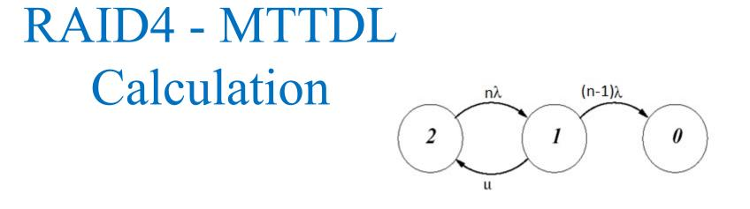
RAID 4/5: data is lost if the second disk fails before the first failed (any one of n) could be rebuilt.
