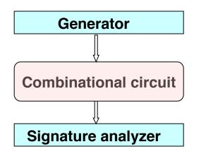
ALFSR: autonomous linear feedback shift register. Better generators include our antirandom test generator.
