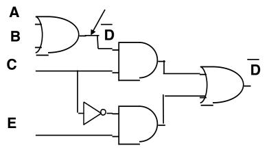
Single path propagation attempts to propagate error using a single path from the fault site to an output.
