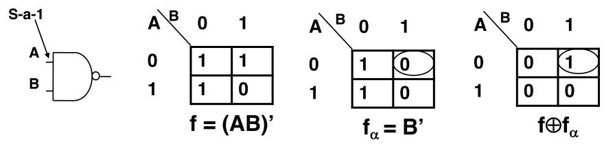
T = A'B (01) is a test. The only test.
