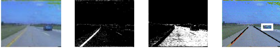
Figure 8: Representative results for MDT-based classification for lane-markers and obstacles (left to right) – original color image, classification for lane-markers, classification for road, obstacles and lanes extracted.
