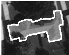
Fig. 4. The middle ROI from Figure 3 after refinement via segmentation [10] and the Generalized Hough Transform [5].
