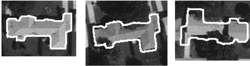
Fig. 3. A demonstration of dynamic control: the three ROIs above were all created by rotation-free correlation, yet the best strategy for refining these hypotheses depends on the quality of the ROIs, not the history of how they were created. In this case, the best strategy is to 1) accept the ROI on the left, 2) reject the ROI to the right, and 3) refine the ROI in the middle through segmentation [10] followed by the Generalized Hough Transform [5].
