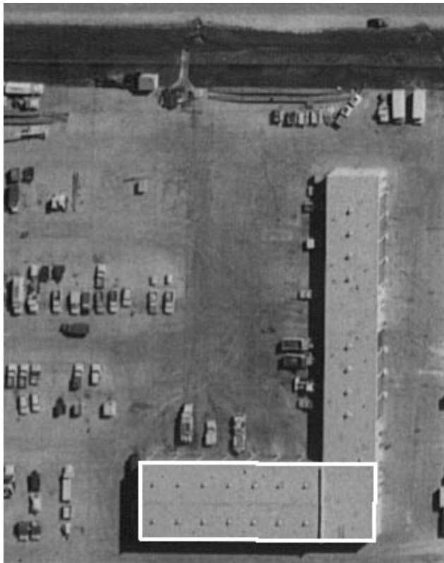
Figure 1: One of the ten aerial images of buildings at Ft. Hood, and the roof hypothesis (shown in white) SLS learned to find in it.
