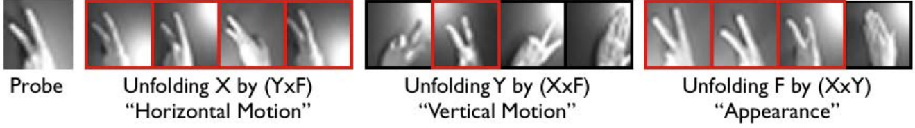
Figure 2. Top 4 neighbors, sorted left to right, from three trees of a Subspace Forest. Those matching the probe class are outlined in red. Samples are from the Cambridge Gestures data set [8]. The “Vertical Motion” unfolding, represented by the second tree, cannot distinguish left-moving from right-moving gestures.
