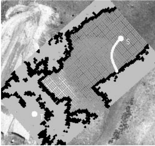
Figure 2: Planning a path for RSTA from (S) to a location on the visibility boundary (shown in black) of a target (T).
