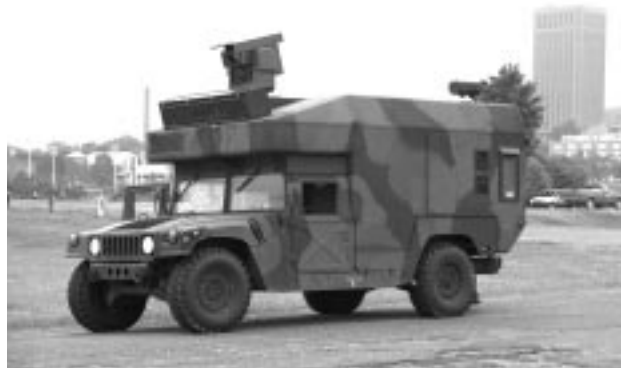
Figure 1: The Mobile Perception Laboratory, built on a modified HMMWV chassis, has computer controlled steering, throttle, and brakes, a complete research laboratory on the back.
