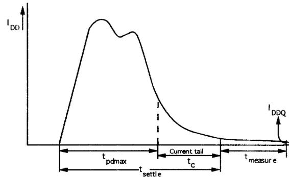
Figure 2: Plot illustrating  $I_{DD}$  vs. Time for a CMOS circuit
