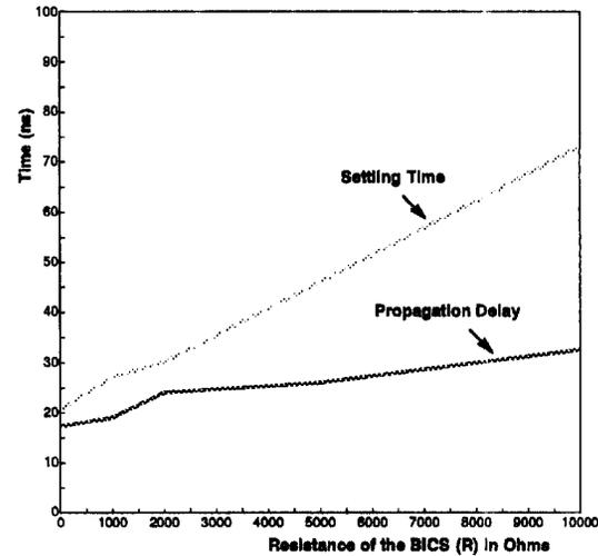
Figure 8:  $I_{DDQ}$  settling time & Propagation delay vs. BICS Resistance ( $R'$ )
