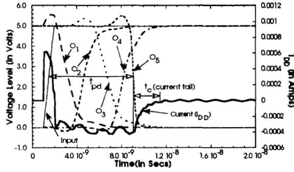
Figure 4: Input/Output & current waveforms for inverter chain with 5 inverters
