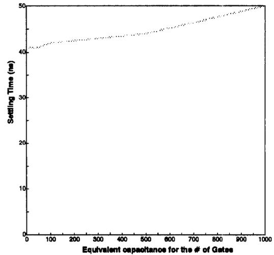
Figure 7:  $I_{DDQ}$  settling time vs. Equivalent Capacitance ( $C$ ) for # of gates
