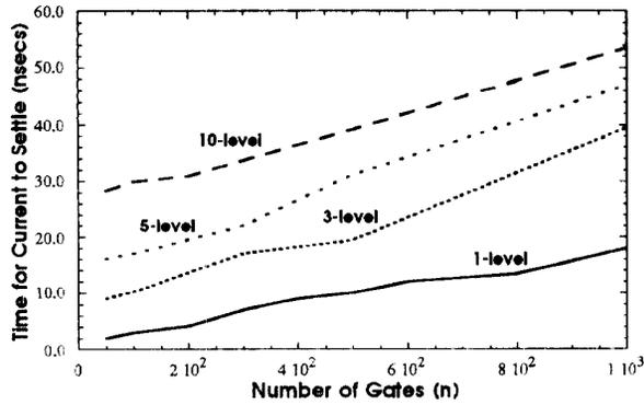
Figure 6:  $I_{DDQ}$  settling time vs. Number of gates for different levels
