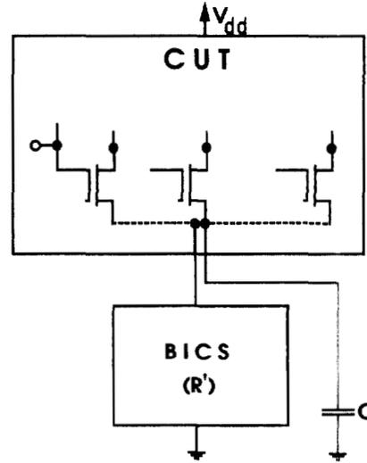
Figure 5: CMOS circuit with BICS
